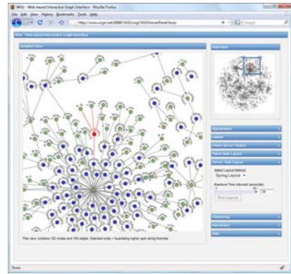
Fig. 2. A screenshot of WiGis displaying results expanded from the seed query "Graph Visualization" on the Citeseer dataset. Graph shows 1104 author and article nodes, with 1125 associations. An overview window of the entire graph is shown in the top right corner with the detail view highlighted by the zoom box.
